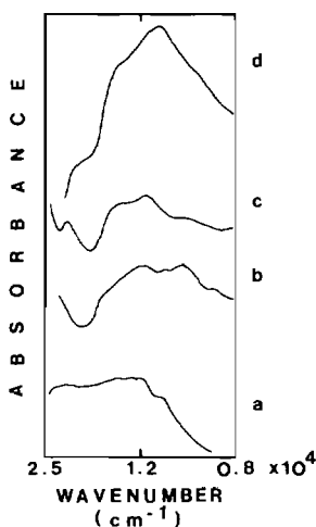
Fig. 1. Diffuse spectroscopy of Mo oxides obtained using HCl as a catalyst at: (a) 25, (b) 300, (c) 600, (d) 900 °C; all for a 72-h period.
